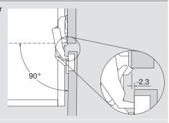
NOTE: Use of 0 mm or 3 mm is recommended for zero protrusion
